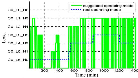
Fig.4. Real and modified modes of fans.
