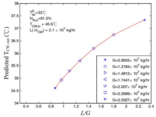
Fig.6. LMN predictions for  $T_{CW,out}$  vs. the water/air mass flow ratio.
